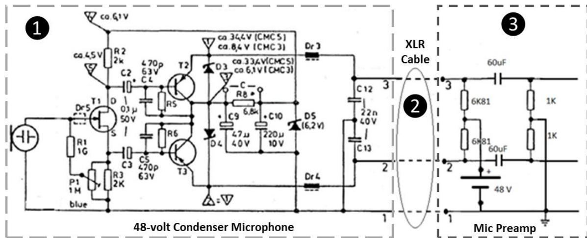
Figure 1. Complete microphone system.
