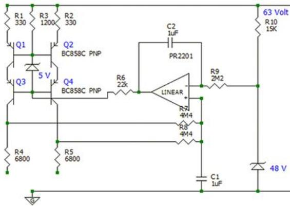
Figure 2. Current-source design – True Phantom.
