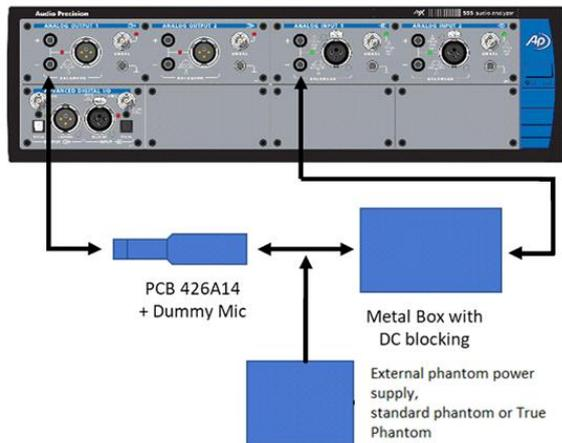
Figure 4. Test Setup
