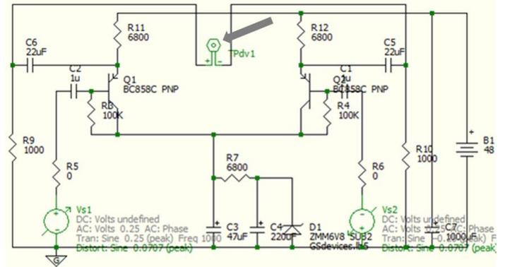
Figure 3. Circuit being modelled using SPICE
