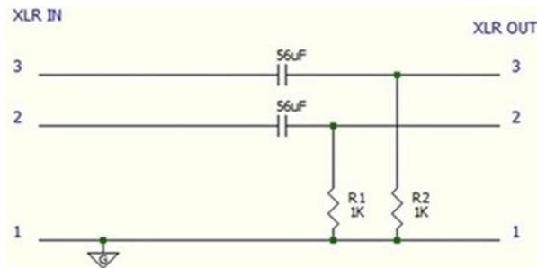
Figure 5. Schematic of DC-blocking circuit
