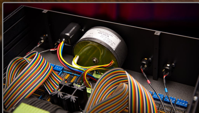
Power module with custom built transformer
