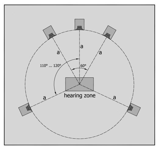
▶ Distance between speakers and your listening position  $a = 0.6 \, \text{m} \dots 2 \, \text{m} (1'12'' \dots 6'7'')$  In case installation in the prescribed way is not possible in your listening room most decoding devices allow adjustments of single speakers.
