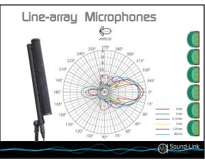
This shows the very narrow vertical polar-pattern of the linearray microphone.
