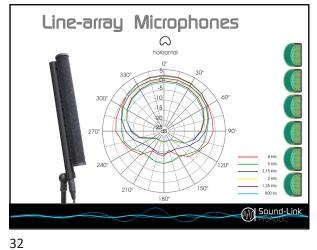
This polar-diagram shows the cardioid horizontal polarpattern of the line-array microphone.
